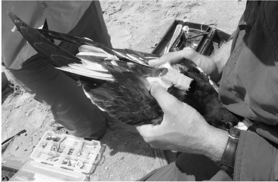
Figure 3.2. Data logger on a Black Skimmer showing the Tesa® tape attachment method.
